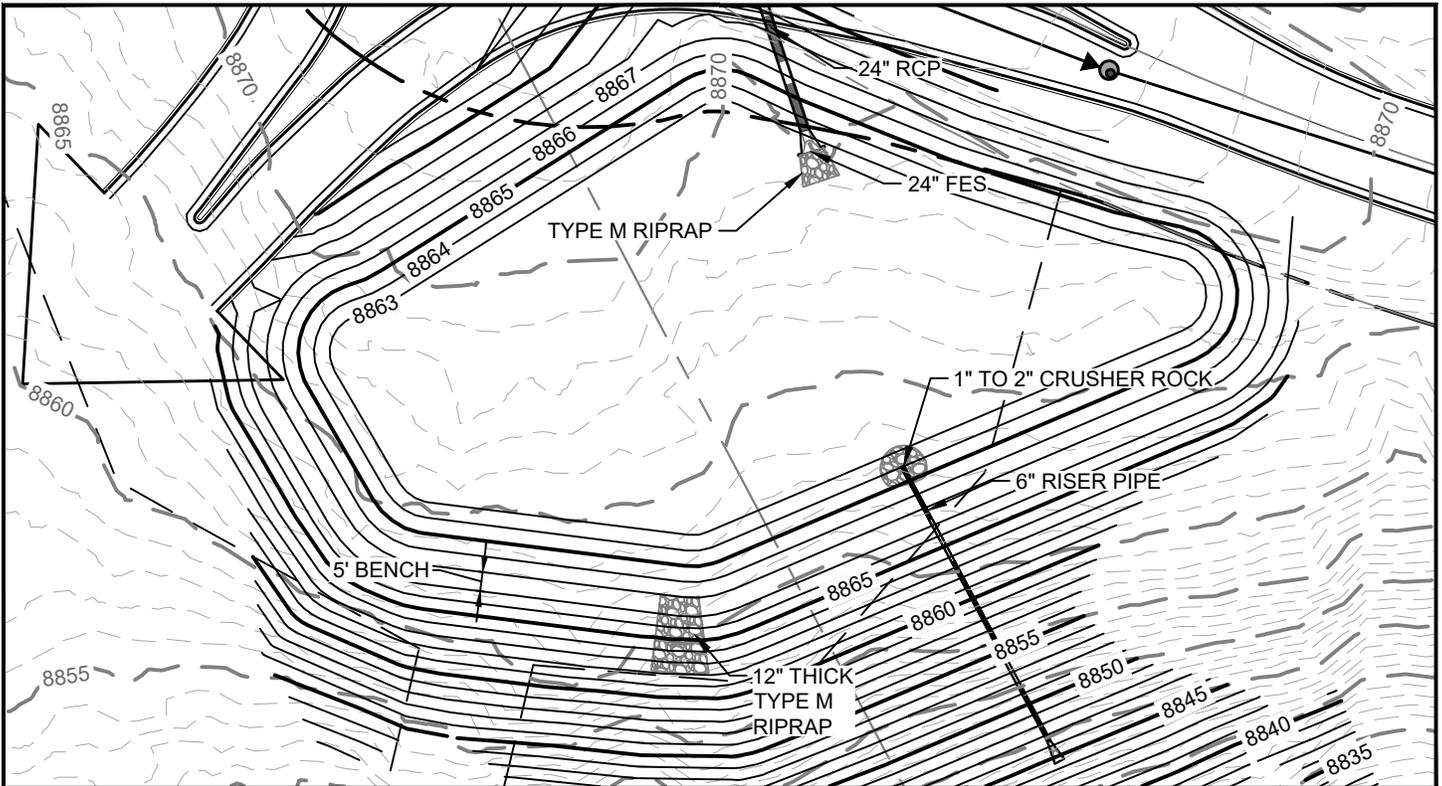
**TEMP SED POND VOLUME CALCULATION PER MHFD DETAIL SC-7**
