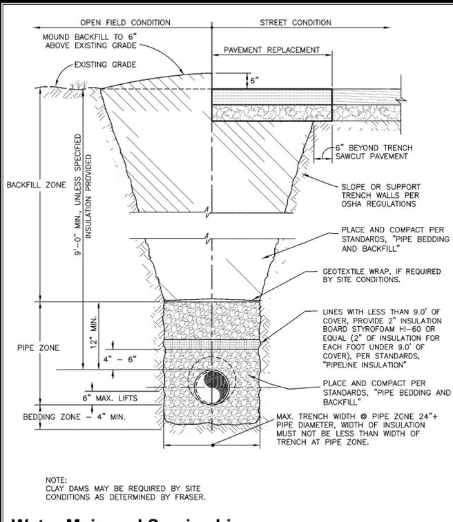
**Water Main and Service Line Bedding and Backfill Detail**
