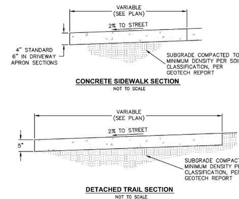
**CONCRETE SIDEWALK SECTION**
